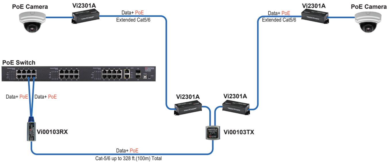
Ethernet and PoE extenders can be used along with the Vi00103 to extend Ethernet and PoE connections. They can be placed on either the switch side or camera side.
