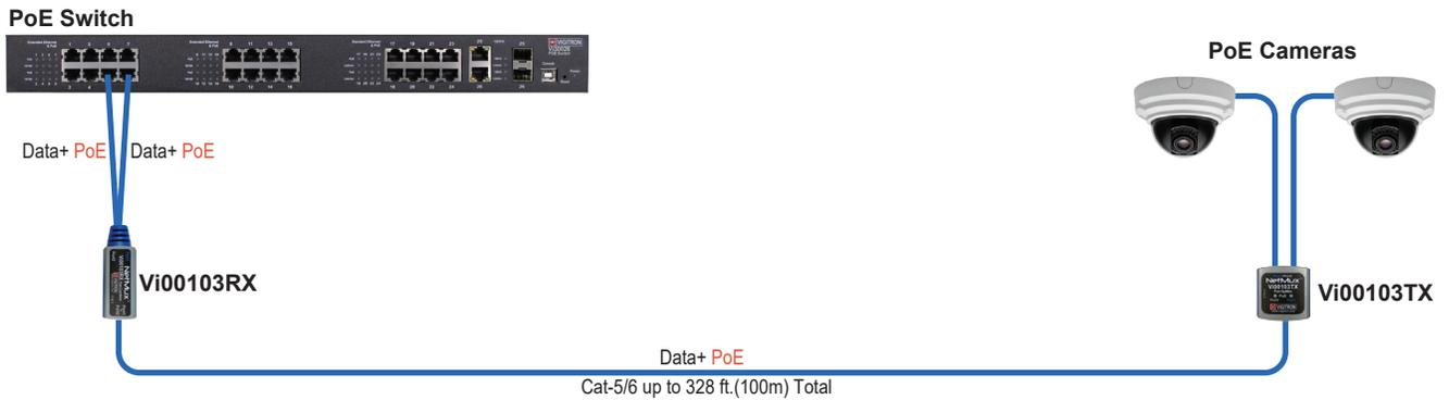
The Vi00103 enables adding an extra PoE camera connection using an existing Cat5/6 cable.
