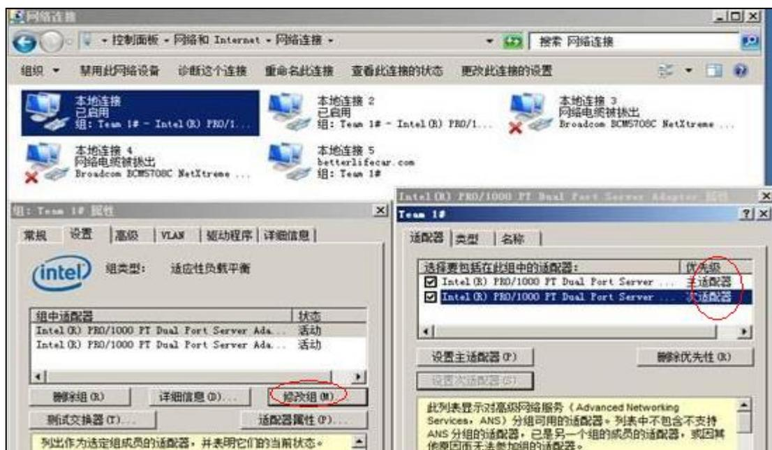
Step 7 Configure IP address for new NIC (Team 1#). IP addresses of the two NICs in teaming cannot be configured.
