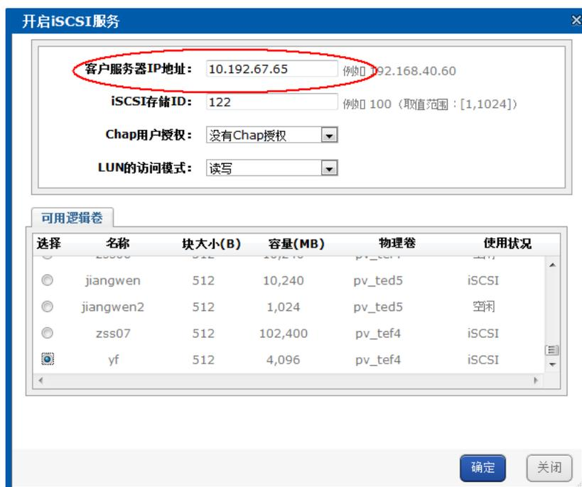
Step 5 If Chap is not enabled in iSCSI target, **Advanced** is not required to click in **Step 8** in 4.1.2 Connect iSCSI initiator to iSCSI target, and **Step 9** can be skipped.
