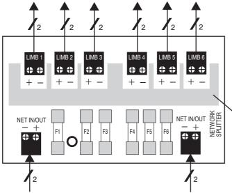
2 CORE SPINE CABLING (e.g. 1mm² T&E) from Network Controler to other Network Splitters
